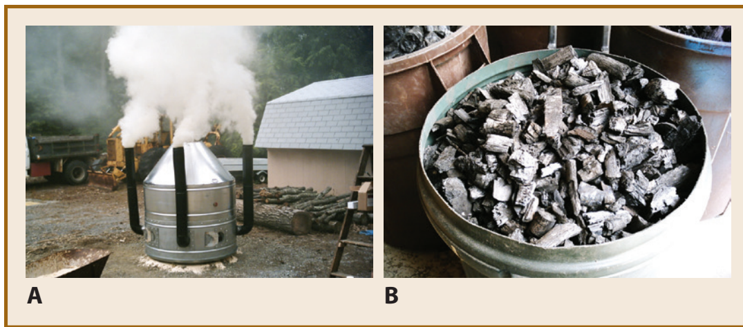
Figure 7: A) Department of Forestry charcoal kiln and B) Ailanthus charcoal.
